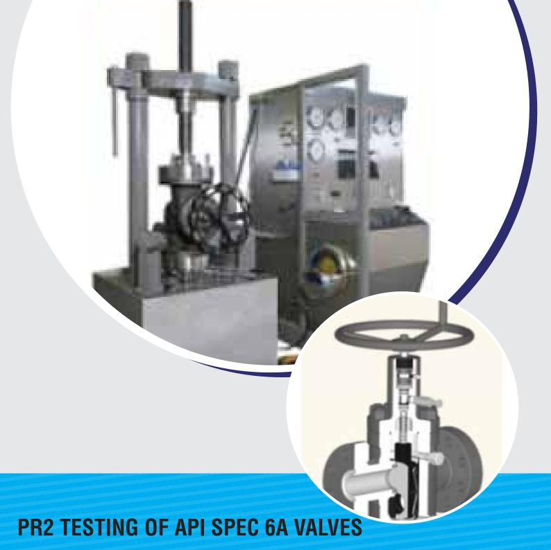
PR2 TESTING OF API SPEC 6A VALVES ANNEX F - DESIGN VALIDATION PROCEDURES - API SPEC 6A PERFORMANCE REQUIREMENT 1 & 2 TESTING OF API SPEC 6A VALVES
